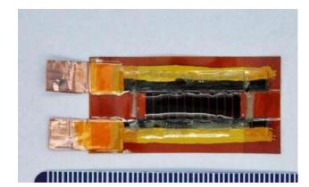
By using lasers to burn electrode patterns into sheets of plastic, manufacturing costs and effort drop massively. The result is a battery that can charge 50 times faster than current batteries and discharge even slower than current supercapacitors. They're even tough, able to work after being bent over 10,000 times in testing.
